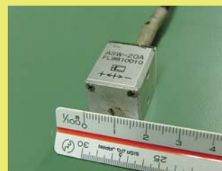
System with Two Accelerometers for Measuring Profile Enabling Real-time data collection
